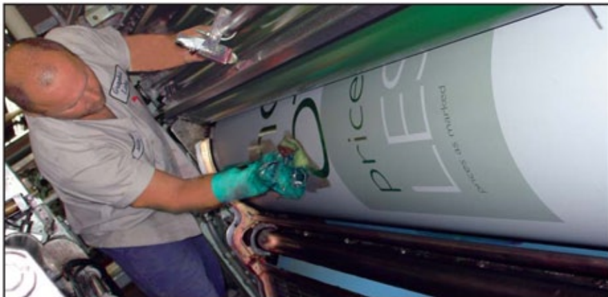
Mike Lawson has a good look at a mounted plate on the five-color Harris press.
