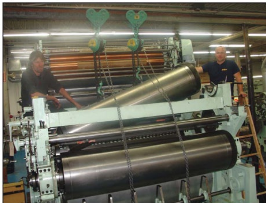
A blanket cylinder is being lowered into position during the installation of the new 54 by 77-inch six-color Harris press.
