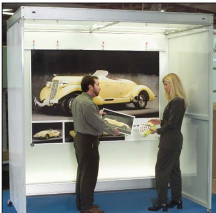
Two Graphic Litho customers stand inside the company's 5000 Kelvin viewing booth. The booth is needed to inspect the company's large format work.
