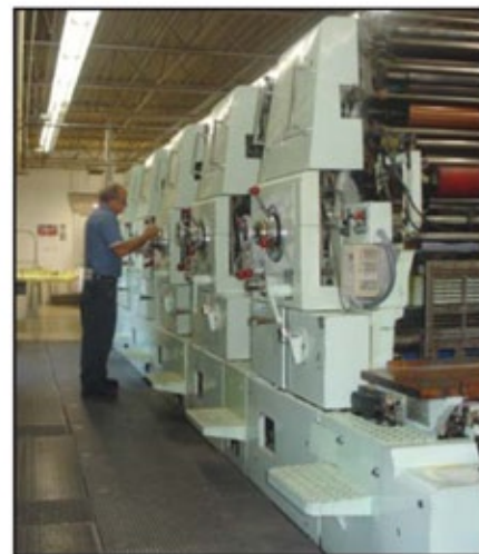
Assistant Pressman Butch Bakeman adjusts settings on the five-color Harris press.
